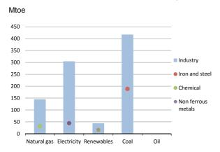
Figure 9. Industry energy consumption by source and sub-sector: 2000-2017 change
