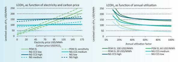
Notes: PEM EL = proton exchange membrane electrolyser; LCOE = levelised cost of energy; NG = natural gas; for the lefthand graph, annual loads of 85% are assumed for all technology options, and the dashed line marks the sensitivity of LCOE for hydrogen from a PEM electrolyser with a 30% variation in cost and a 10% variation in efficiency.
