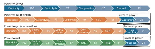
Note: The numbers denote useful energy; except for gas turbines, efficiencies are based on HHV; the conversion efficiency of gas turbines is based on LHV.
