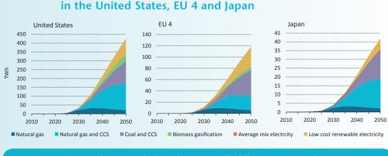
Figure 17: Hydrogen generation by technology for the 2DS high H<sub>2</sub>
